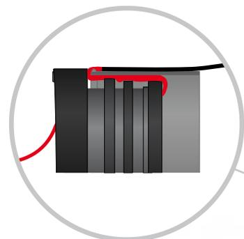
The red area illustrates the seal pinned in between the PU-ring (light grey) and the Oval Stiff Ring.
