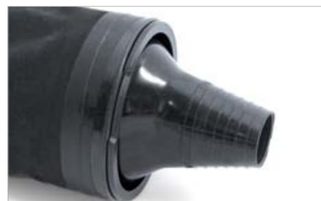
**2.5** Make sure the Oval Stiff Ring is bottomed out and that the Ring flange is in the position shown in the image. Before diving your ANTARES system, you should check that the Oval Stiff Ring and seal has been fixed correctly in position. Grab the seal with one hand and try to pull it in the opposite direction from the suit without using excessive force. If everything feels ok, perform test dive! If not ok, refer to images **1.3-1.4**.
