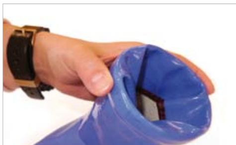
**4.2** Fold the glove shaft inwards over the Oval Spanner Ring, (latex gloves can be fitted and folded the opposite way).
