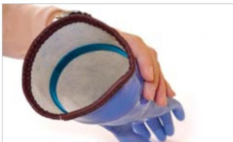
**4.1** Place the Oval Spanner Ring on the inside of the glove. Make sure to find proper position for optimized length and ergonomics.
