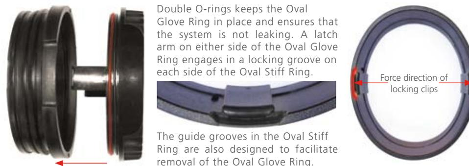
Double O-rings keeps the Oval Glove Ring in place and ensures that the system is not leaking. A latch arm on either side of the Oval Glove Ring engages in a locking groove on each side of the Oval Stiff Ring.
