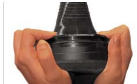
**2.3** Squeeze the two rings together, make sure that the seal does not slide out of its position.
