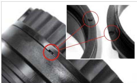
**5.5** Check the fittings between the Oval Glove Ring and the Oval Stiff Ring. Ensure the latch arms have locked into the locking grooves and that the alignment nuts has positioned itself in its alignment grooves.
