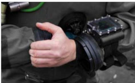
**5.4** Press the Oval Glove Ring into the Oval Stiff Ring on both sides until you see that it has bottomed and is properly fitted.
