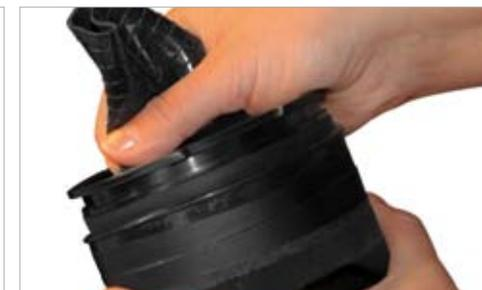
**2.2** Keep the seal in a fixed grip and rest the Oval Stiff Ring firmly against your hand, when pressing the rings together. This will prevent the seal from slipping out of position.
