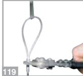
Tie, using a fishing-line clip and a pair of pliers, the line to the rear hole of the spear making a loop about 60mm long (119).
