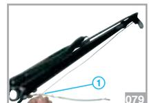
Put the loose end of the fishing-line in the loop of the line-tension system and make a loop, using the second fishing-line clip (080-1).
