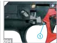
In this event, if you load the spear in the handle, the trigger-mechanism will not hold it. To solve the problem, remove the spear and pull the trigger a couple of times before reinserting the spear. The pawl will return to the correct position.
