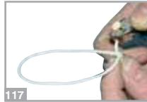
Make a loop at each end of the line-tension system (115). Cut the excess line, at a distance of 5-10 mm from the knot, using a pair of scissors (116) and burn the cut end with a lighter to
