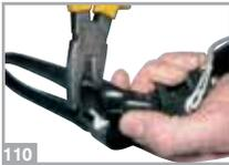
Remove the wishbone and unscrew the rubber-slings from the muzzle. The slings are tightly screwed on the muzzle for safety reasons so; if you cannot screw and unscrew them by hand, use a pair of pliers placing it on the plastic ring (**110**).
