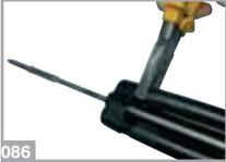
Remove the wishbone and unscrew the rubber-slings from the muzzle. The slings are tightly screwed on the muzzle for safety reasons. If you cannot screw and unscrew them by hand, use a pair of pliers placing them on the plastic ring **(086)**.
