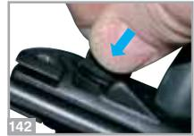
Guide, then, the ring inside the socket ensuring that the groove meets the protuberance at the socket's interior. From this position, holding the sling from as close to the ring as possible (**142**), push it inside the socket. You will hear a characteristic 'click' indicating that the ring has locked in the muzzle and the rubber-sling is firmly held and cannot move loosely in the muzzle.
