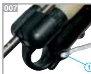
**AMI muzzle.** This muzzle takes one pair of screwed rubber slings and has a holder for a single circulated rubber sling. The thread of the sockets is M14x1. The muzzle has an opening to hold and direct the spear. It also has a  $\Phi 4$  hole (007-1) to fasten line-tension system.
