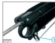
**Articulated VELOS muzzle.** This is a two-part muzzle with an articulation. It consists of a base (009-1) and a moving part (009-2). It takes one pair of screwed rubber slings and has a holder for a single circulated rubber sling. The thread of the sockets is M14x1. It features an adjustable opening to hold and guide the spear. It has a fitted metallic guide (010-1) to fasten the line-tension system or to direct line of the reel when one is used.
