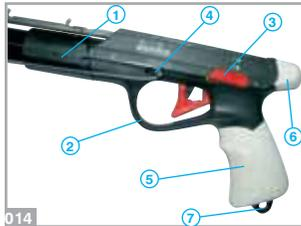
This handle has cassette-type trigger and trigger-safety mechanisms and an extended covering part of the handle (014-1). It has a trigger-cover (014-2), a safety lever (014-3), a line drop mechanism (014-4) and an extra clip (015-1) to hold the line. It features a soft cover (014-5) on the sheath and a soft heel (014-6) to ease the pressure on the user's body during arming. A hole at the bottom of the sheath serves to hang the speargun from the buoy (014-7).
