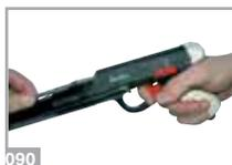
The spear is placed in the speargun by the manufacturer. To remove it, hold the handle and press the trigger pulling at the same time the spear outwards with your other hand **(090)**. You will hear a characteristic 'click' when the spear is released by the trigger-mechanism.
