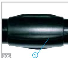
**ALS  $\Phi 28$  spear-guide.** Internal diameter  $\Phi 28$ . It guides the spear during the shot. By rotating it or moving it along the barrel, it is possible to adjust the shot to the personal preference of the user. It has fins on its two sides (005-1), which allow the neat placement of
