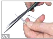
Make a loop at each end of the line-tension system (071). Cut the excess line, at a distance of 5-10 mm from the knot, using a pair of scissors (072) and burn the cut ends with a lighter to prevent them from fraying (073).
