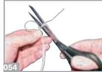
Cut the excess line, at a distance of 5-10 mm from the knot, using a pair of scissors (054) and burn the cut ends with a lighter to prevent them from fraying (055).
