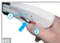
The safety is deactivated in position (045-1). If the speargun is armed and you pull the trigger, the spear will be released and launched. To activate the safety-mechanism, press the red button (045-2) until it comes out from the other side of the handle (046-1). When the safety is in this position (046-1) the trigger is blocked and cannot be pulled to release the spear.
