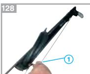
For having a line length three times the barrel length do the following. Put the line through the line drop mechanism, bring the loose end to the muzzle and cut the line at that point (128-1).
