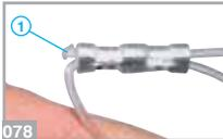
Cut the excess fishing-line, at a distance of about 4-5mm from the fishing-line clip, with a pair of scissors (076). Burn carefully the cut end with a lighter (077) and, while it is still soft shape it into a small head (078-1) using wet fingers.
