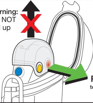
Pull forward only to remove antenna retainer
