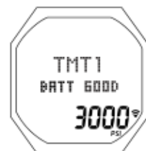
Fig. 60 - TMT BATTERY STATUS
