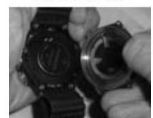
Fig. 179B - LIFTING BATTERY COVER OFF
