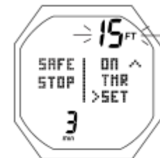
Fig. 46B - SET SAFETY STOP (set Time then Depth)
