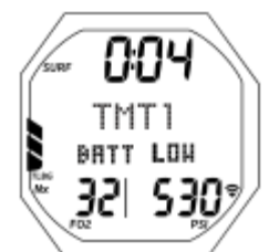
Fig. 2 - TMT LOW BATT ALARM (Surface Main)
