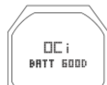
Fig. 59 - OSi BATTERY STATUS
