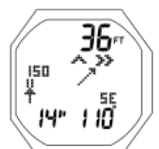
Fig. 163 - REF OP MAIN (at 110°, turn right to 150°)
