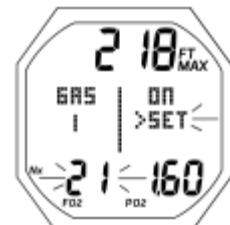
Fig. 30B - SET GAS 1 (to set FO2 then PO2 alarm)
