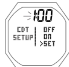
Fig. 6C - SET CDT (hour then minutes)
