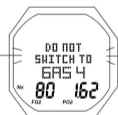
Fig. 101 - GAS SWITCH ALARM
