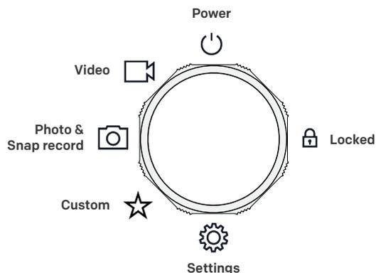
You can select mode by rotating the ring and align the mode with the logo plate.
