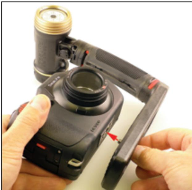
Align the underwater camera to the light's mounting screw and hand-tighten.
