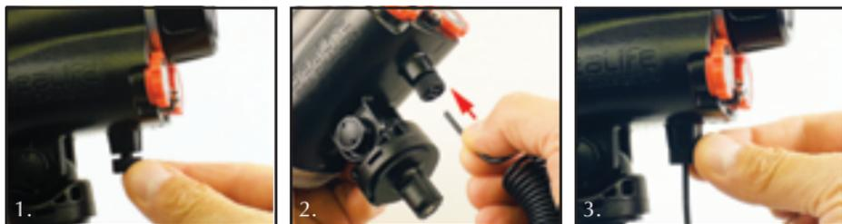
1. Turn the cable locking screw counter-clockwise by about 2 rotations to loosen the clamping effect of the lock. Do not remove the locking screws.
