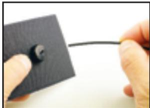
**Step 5:** Insert the cable(s) so about 1mm sticks out of the other end and tighten the cable adapter assembly. Hand tighten – do not use tools. .
