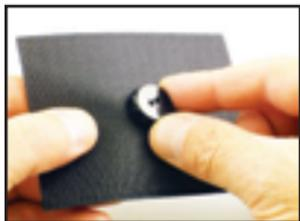
**Step 4:** Loosely screw on the smaller half of the adapter.
