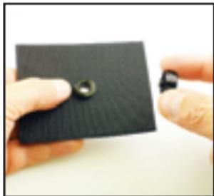
**Step 3:** Unscrew cable adapter assembly and insert the larger half through the hole of the hook-n-loop fastener as shown. Make sure the “hook” side of the fastener is facing towards the wide end of the adapter (towards the camera).
