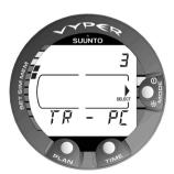
**Fig. 4.15 Data Transfer Mode.** [3 TR-PC].
