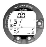
Fig. 3.21 Surface display in the NITROX Mode.
