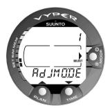
Fig. 4.24 Altitude Adjustment and Personal Adjustment Setting Mode. [1 AdJ MODE]. To enter the Altitude Adjustment and Personal Adjustment Setting Mode select MODE- 3 SET-1 SET DIVE- 1 AdJ MODE (Fig. 4.24). Now you are able to select from the three altitude modes (Fig. 4.25) and the three personal modes (Fig. 4.26).
