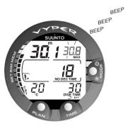
Fig. 3.33 Preset maximum depth alarm is activated.
