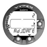
Fig. 4.36 Adjust Date Setting Mode. [2 AdJ DATE].
