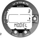
Fig. 4.45 Dive ComputerModel Setting Mode.[3MODEL].
