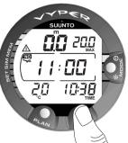
Fig. 3.29 Surface interval, noflying time. Pressing the TIME button twice will show the no-flying time, indicated by an airplane symbol.
