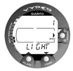
Fig. 4.41 Backlight Setting Mode. [1 LIGHT].
