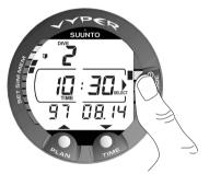
**Fig. 4.11 Logbook, page I.** Press the SMART (Select) button once to be able to scroll between the different dives.
