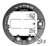
Fig. 4.30 Setting The Maximum Depth Alarm. Press the scroll buttons to change the alarm on/off and to set the maximum depth value.
