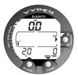
**Fig. 4.18 Selected Dive Simulator Mode.** Descent by pressing the arrow down (TIME) button and ascent by pressing the arrow up (PLAN) button.
