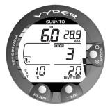
Fig. 3.10 Ascent rate indicator. Two segments.
