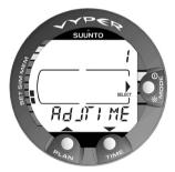
Fig. 4.34 Adjust Time Setting Mode. [1 AdJ TIME].
