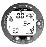
Fig. 3.30 Surface Mode after a violated decompression dive. The Er symbol indicates that you have violated the ceiling for more than three minutes. You must not dive again for at least 48 hours.
