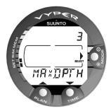
Fig. 4.29 Maximum Depth Alarm Setting Mode. [3 MAX DEPTH].
