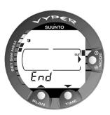
Fig. 4.12 Logbook, end of the memory. The END text is displayed between the oldest and the most recent dive.
