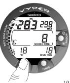
Fig. 3.9 Diving display. An annotation, Bookmark, is done in the profile memory during a dive by pressing the PLAN button. Note the Logbook symbol.
