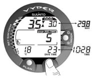
Fig. 3.18 Decompression dive, at the ceiling zone. The two arrows point at each other ("hour glass"). You are at the optimum ceiling zone at 3.5 m [11 ft] and your minimum ascent time is 5 minutes. By pressing the TIME button you can display maximum depth and time.
