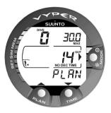
Fig. 3.6 Dive Planning. The Planning mode is indicated by the PLAN text. The no-decompression time limit at 30.0 m [100 ft] is 14 minutes in A0/P1 mode.
