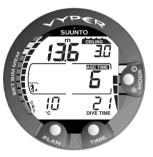
Fig. 3.17 Decompression dive, above the floor. The upward pointing arrow has disappeared and the ASC TIME label has stopped blinking, which means that you are in the decompression range.
