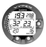
Fig. 3.22 Diving in the NI-TROX Mode. The  $O_2$ % is set to 32%.
