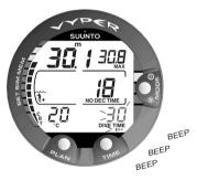
Fig. 3.32 Preset dive time alarm is activated.
