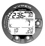
Fig. 3.16 Decompression dive, below the floor. The upward pointing arrow and the blinking ASC TIME label tell you to ascend. The minimum total ascent time including the safety stop is 7 minutes. The ceiling is at 3 m [10 ft].
