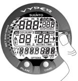
Fig. 3.1 Startup I. All segments shown.
