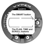
Fig. 2.2 The push buttons of the dive computer.
