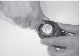
Fig. 5.2 Opening of the securing ring.
