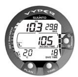
Fig. 3.12 Ascent rate indicator. Four segments.
