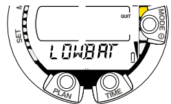
Fig. 3.2. Startup II. Battery power indicator.
