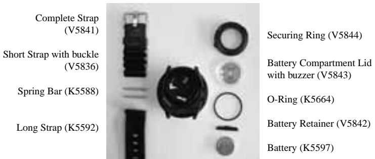
Fig. 5.1 Instrument parts. The code after the name stands for spare part order number.
