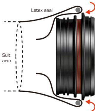
**1.** Start by removing the Silicone groove ring from the middle groove.
