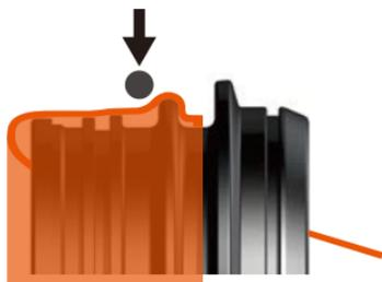
**2.** Pull the seal back until the ridge is all the way down to the o-ring.
