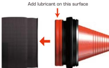
**5.** Twist the seal and pull it back with your hand during the mounting procedure to avoid wrinkles.
