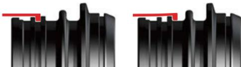
**4.** Add some waterbased lubricant on the Silicone section that slides into the suit arm. Make sure the Silicone doesn't wrinkle when pushing it into the suit.
