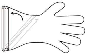
**2.** Mount the o-ring in the groove.
