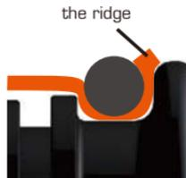
**3.** Pull the drysuit Latex seal over the Silicone seal and onto the suit ring. Check the seal is centered. Mount the o-ring into the deep groove.
