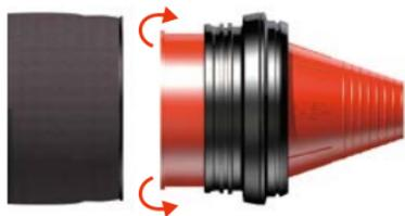
**3.** The ridge on the seal should be placed in the second groove as standard. (In some cases it can be placed in the next groove to achieve better sealing)
