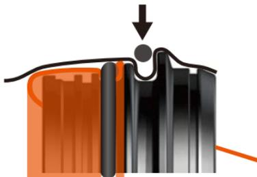
**4.** Fold back the remaining part of the latex seal as shown in the image.
