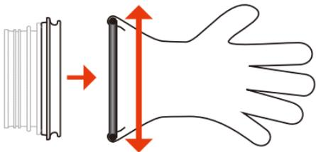
**3.** Check the glove is correctly mounted and is the desired length.
