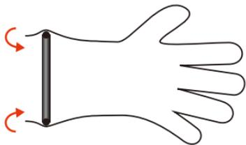
**2.** Open the glove and o-ring by pulling with both hands firmly and mount it onto the glove ring.
